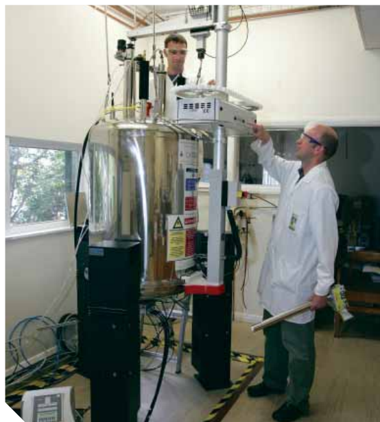
Gavin Painter (left) and Phil Rendle use IRL's recently upgraded 500 MHz NMR spectrometer to analyse adjuvant samples.
