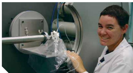
IRL Research Scientist Bridget Ingham mounts a flow cell in place for the first general user experiments using the powder diffraction beamline at the Australian Synchrotron.
