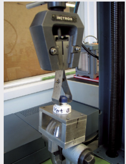
Vertical pull-off test (Photo courtesy EverEdge IP)
