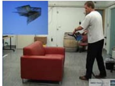
Above: IRL's 3D scene-scanning technology in use. The operator works much like a spray painter, progressively covering the scene and recording the 3D data as a computer file.
